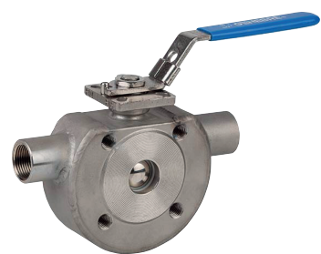
Art. 2119 Wafer type - 1Pc full bore ball valve with heating chamber. Mounting between flanges PN 16
